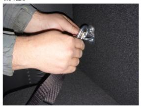
Note: If the seat does not want to catch, you may have to pull the strap away from the middle of the seat latch. You may have to use force to latch the seat which will also tighten the strap.
