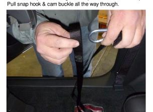
4 Pull snug to tighten the Vault to the floor of the vehicle. Fold seats back into the normal position.
