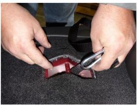
3. Hook the end of the snap hook onto the D-ring on the back of the Vault.
