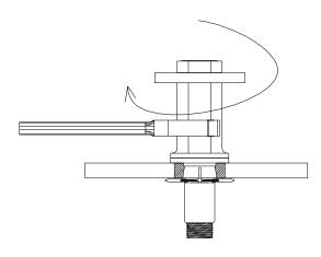
11 Attach 5/16" fender washer & flare tool onto 2" bolt and thread into Plus-Nut
