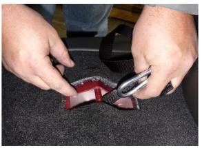
3. Hook the end of the snap hook onto the D-ring on the back of the Vault.
