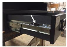
2. Open the lid of the cargo storage tray. Remove the rubber mat & hold down bolts in the bottom of the tray. Relocate the jack from it's storage compartment on the drivers side cargo panel. The truckvault will block the access to this panel.
