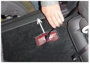
Note: Specific installation may vary according to your model of Vault and vehicle make, model and year. Use whichever method gives you the easiest installation while providing the most secure and safe attachment. The Vault should be sturdy & the straps tight at the end of installation. Please call us with any questions or concerns.
