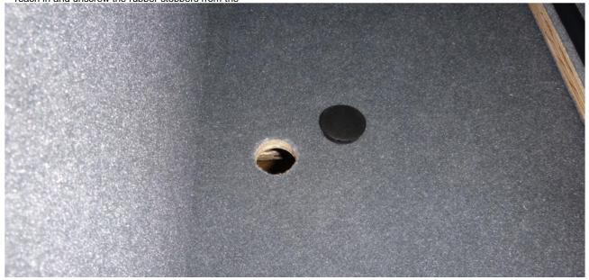
3 Pop the top cover cap out from underneath the top of the TruckVault. Close the drawer and insert the spare access rod through the holes and into the pare tire release. You may have to roatate the tool to line it up with the release. Use the supplied 10mm wrench to lower the spare tire.
