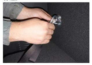
Note: If the seat does not want to catch, you may have to pull the strap away from the middle of the seat latch. You may have to use force to latch the seat which will also tighten the strap.
