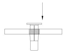
Hold flare tool with 9/16" wrench. Tighten bolt with impact wrench to collapse insert.
