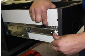
3 Assemble Mounting frame. See the drawing below to build the mounting frame before placing it in the vehicle.
