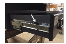
2 Locate and remove the track bolts (A) on the side of the Vault.
