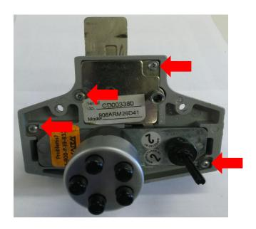
You will then need to remove the button assembly and gear plate from the lock assembly. (Four Screws)
