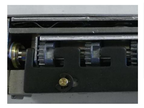
Code gears that have the notch lined up with the tab next to them are NOT part of the combination, these can be ignored.
