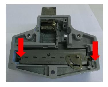
Remove the tumbler assembly. (Two Screws.)
